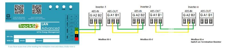
Note: At any one point of time only 1 Modbus Master-TrackSo Datalogger or Inverter Stick can be connected to Inverter for monitoring.
